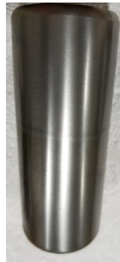
Picture of Blaze coupling post acid test and polishing. No attack was noted.
