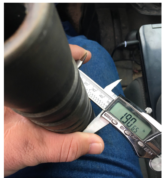
Blaze treated plunger showing less than 0.01% wear on the OD. A new plunger will measure 1.910 in OD.
