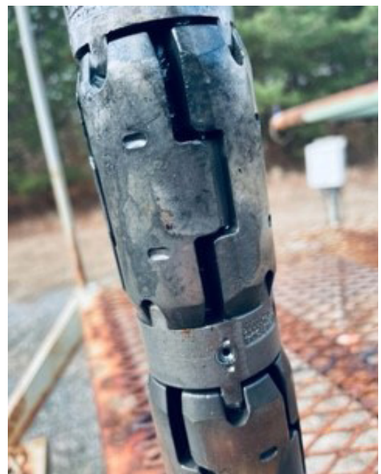
BLAZE-treated plunger after 5+ months of run time. The wear indicators on the pad demonstrate that wear was minimal despite the small decline in production.
