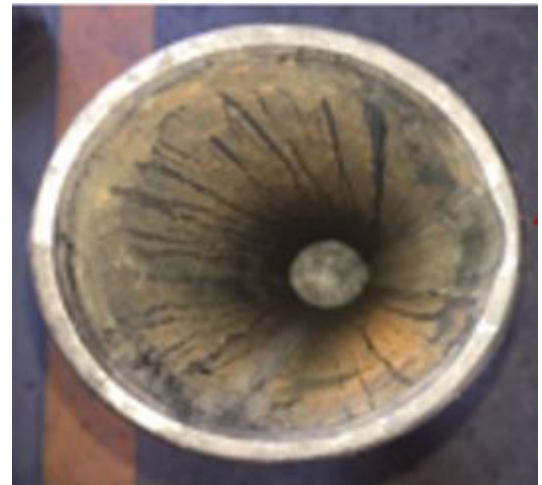
Photo of BLAZE-treated pup joint after 16 month run time.
