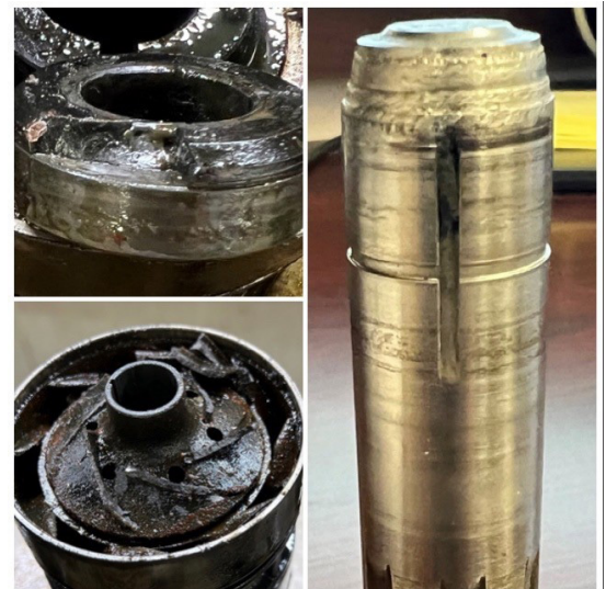
Top Left: Broken TC bearing from top pump. Bottom Left: Damaged stage in top pump. Right: Cut shaft.
