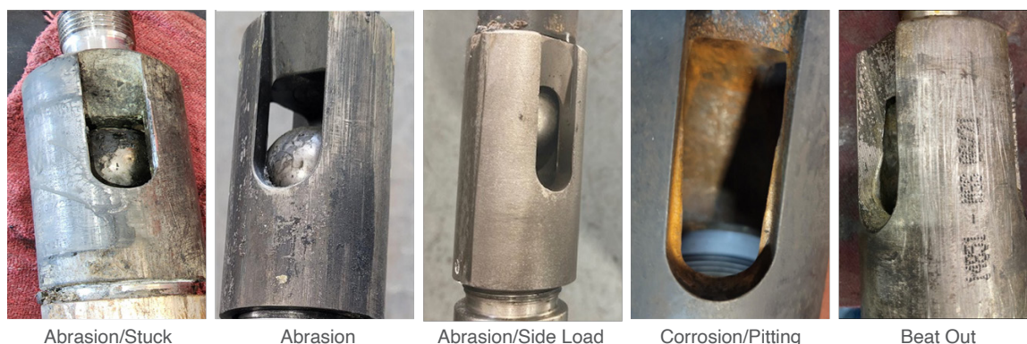
Image 3 Examples of common failure modes of sucker rod pump cages
