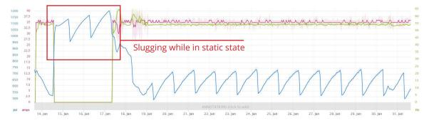
Due to an up-dip horizontal, the well exhibits slugging behavior even in static states. In managing these slugs, the Genesis System proved to be a pivotal component in preventing downtime for the well.
