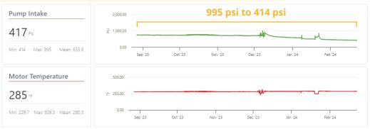
Despite high GOR and gas rates, the Genesis System has achieved a remarkably smooth fluid level drawdown of over 500 psi with minimal motor temp swings and zero gas related shut downs. The well continues to operate in a stable state as of publication.
