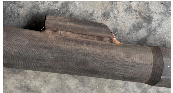
BLAZE treated GL Mandrel showing no corrosion-erosion of the Lug/GLV port after 8.5 month run time.
