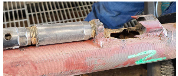
Conventional GL Mandrel showing corrosion-erosion of the Lug/GLV port after 6 month run time.
