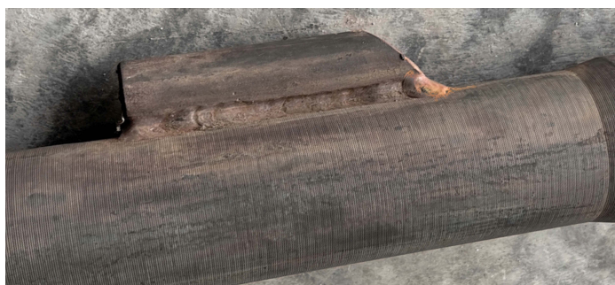
Inspected BLAZE®-treated mandrel at 8-1/2 months
